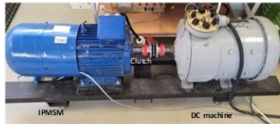
Fig. 12. Photo of experimental stand with the IPMSM clutched to DC machine
