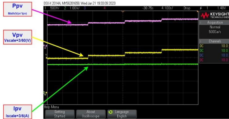
Fig. 15. The response of PV power, voltage and current for different temperature levels obtained by the HIL configuration on the oscilloscope
