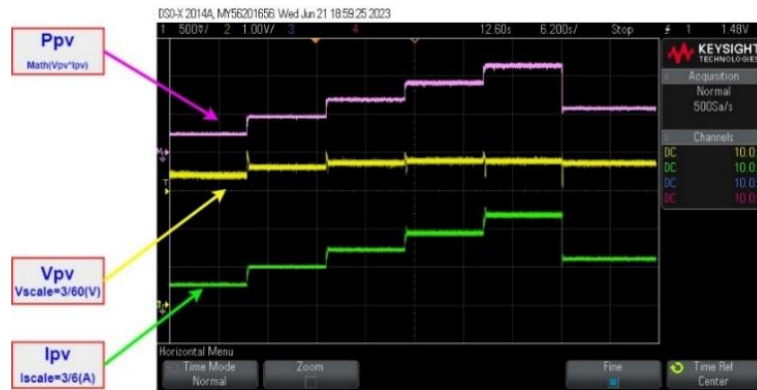
Fig. 13. The response of PV power, voltage and current for different irradiance levels obtained by the HIL configuration on the oscilloscope
