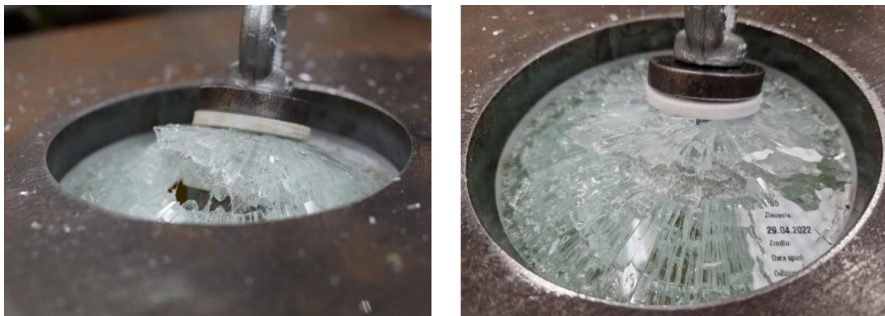
Fig. 10. View of damaged samples – reference sample (left), reinforced sample (right)
