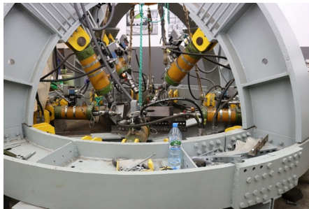
Fig. 3. Test stand for multi-directional strength testing
