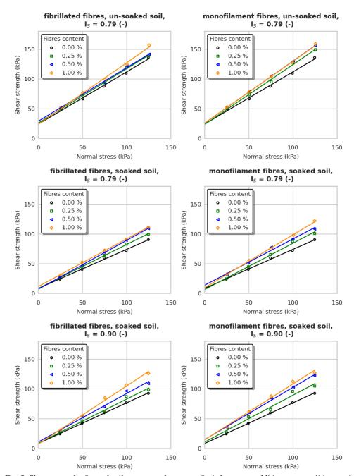
Fig. 3. Shear strength of tested soil vs. type and amount of reinforcement addition, test conditions and degree of compaction
