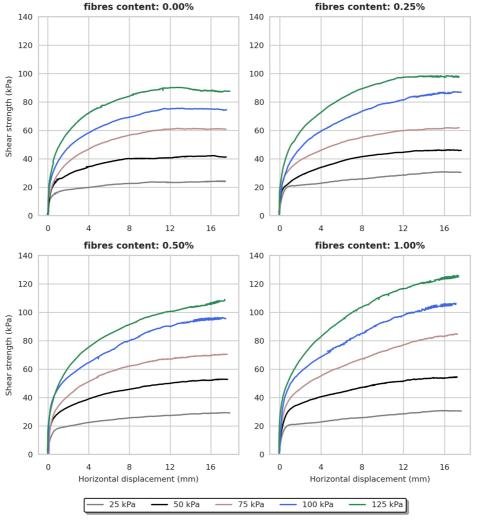
Fig. 2. Shear stress vs. horizontal displacement for unreinforced and reinforced soaked soil samples with a degree of compaction of  $I_S = 0.90$  (results for monofilament fibres)
