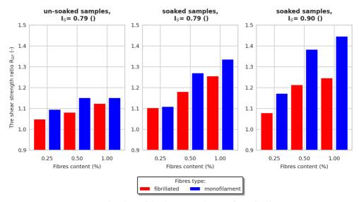
Fig. 4. Values of the shear strength ratio of tested soil
