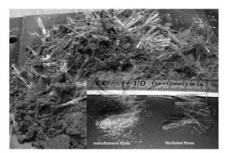
Fig. 1. The view of soil sample reinforcement with fibrillated fibres and the view of both types of fibres used in the tests
