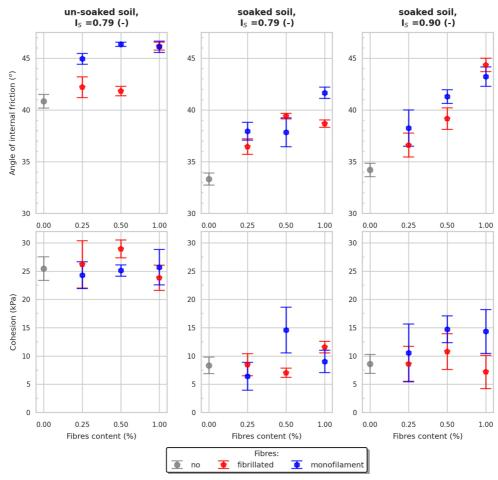
Fig. 6. Values of peak shear strength parameters of tested soil with the addition of polypropylene fibres (vertical bars represent standard deviation of parameter)
