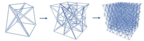
Fig. 1. Tensegrity metamaterial: cell - supercell - lattice
