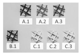
Fig. 3. Series 1 - tensegrity-inspired cell samples
