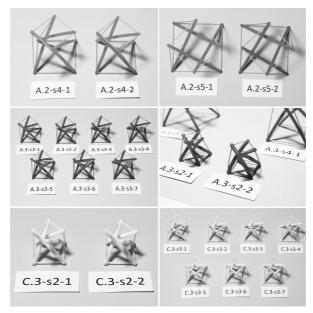
Fig. 4. Series 2 – selected tensegrity-inspired cell samples
