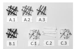
Fig. 7. Series 1 - tensegrity-inspired cell samples after the uniaxial compression test
