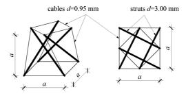
Fig. 2. Geometry of the 4-strut simplex module
