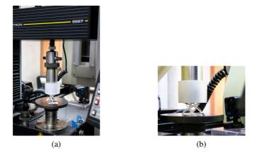
Fig. 5. Test stand: a) universal testing machine with a sample; b) sample under compression
