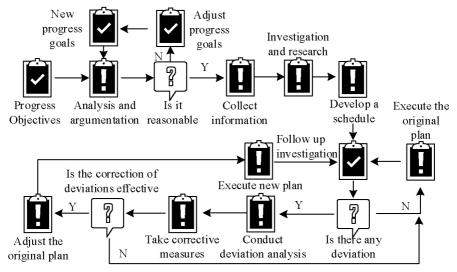
Fig. 1. Construction progress management flow chart
