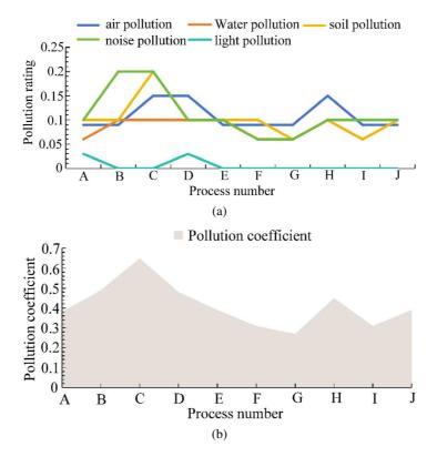
Fig. 6. Construction pollution and proportion of pollution in each process; (a) Pollution ratings for each process, (b) Various pollution coefficients of each process
