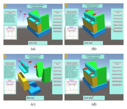
Fig. 8. Display of disassembly and assembly process; (a) Support pad disassembly, (b) Anti vibration block disassembly, (c) Expand All Components (d) Reset
