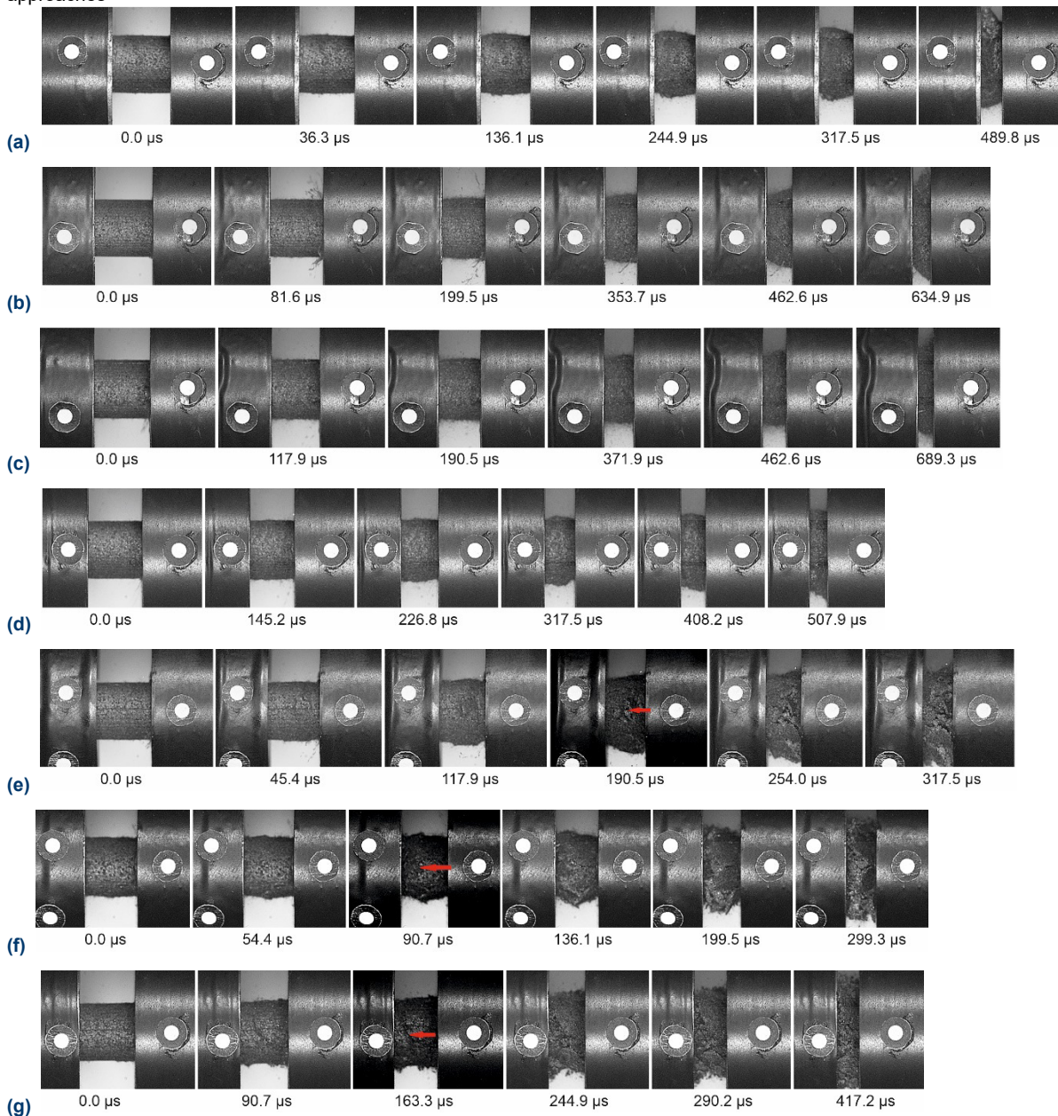
Fig.7. Frames taken from video records of DIHPB tests of: (a) Ti+100AC; (b) Ti64BEPM+50AC; (c) Ti64BEPM+75AC; (d) Ti64BEPM+100AC; (e) Ti64PA+50AC; (f) Ti64PA+75AC; (g) Ti64PA+100AC (Red arrows in (e,f,g) indicates appearance of brittle cracks)
