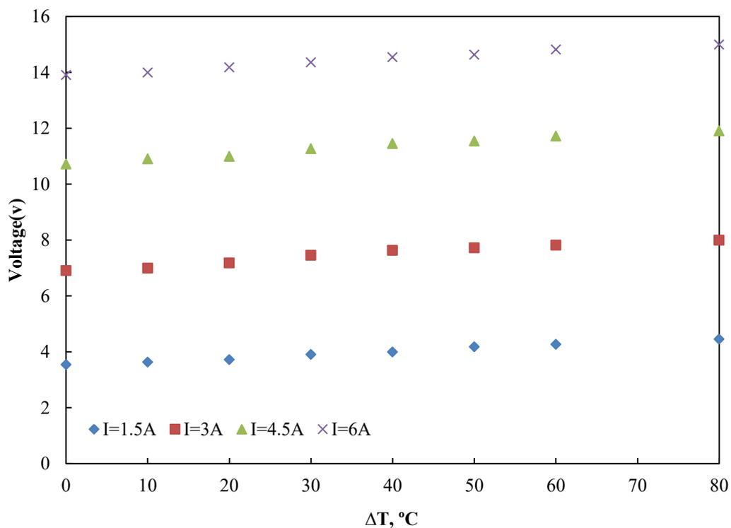
Fig. 3. Performance specification curves  $\Delta T$  vs. voltage for Peltier
