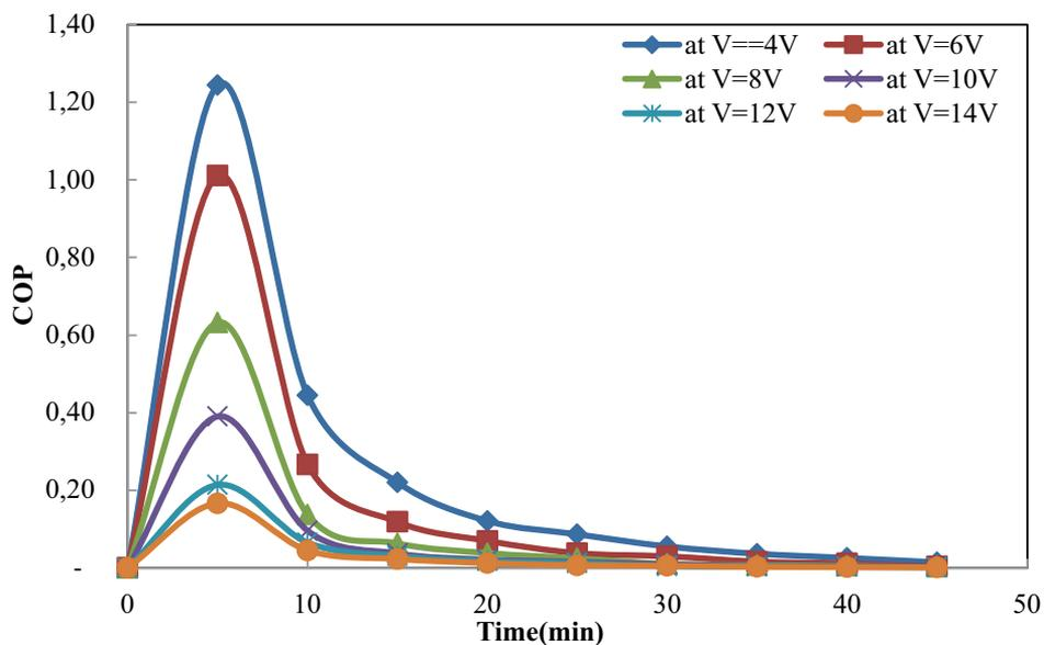
d) Effect of using four Peltier units on COP over time at different voltage
