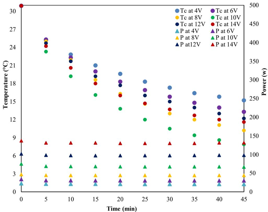
Fig. 8. Variation of temperature and power by using two Peltier units
