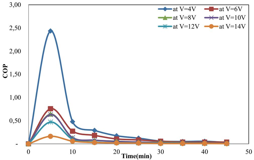
a) Effect of one Peltier on COP over time at different voltage
