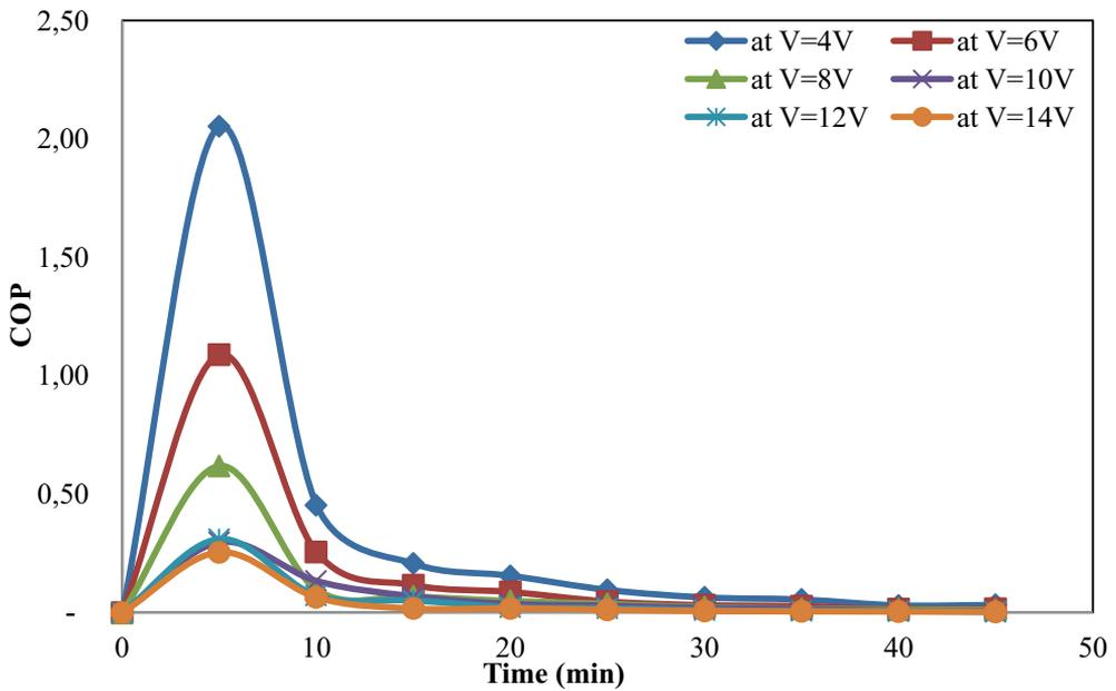
b) Effect of two Peltier units on COP over time at different voltage
