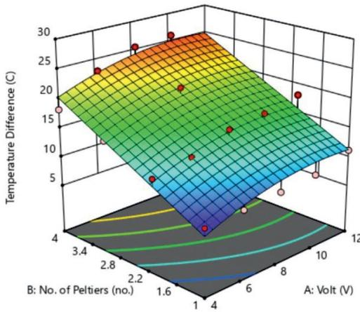
a) Effect of number of Peltier units and voltage on temperature difference
