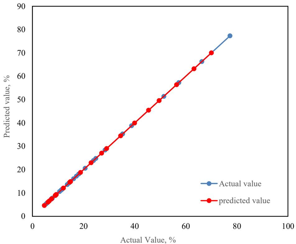
Fig. 5. Actual and predicted values for the cooling temperature difference model
