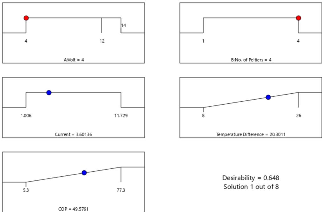
Fig. 13. Maximum temperature difference and COP at optimal experimental factors
