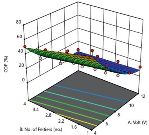
b) Effect of number of Peltier units and voltage on COP%
