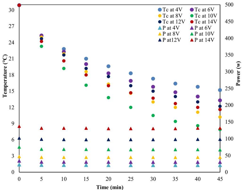
Fig. 9. Temperature and power variations over time for operation with three Peltier units
