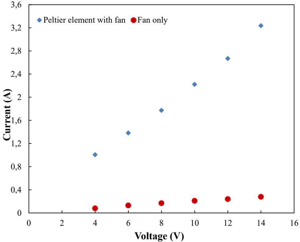
Fig. 4. Relationship between V & I for Peltier unit with fan and fan only at constant time
