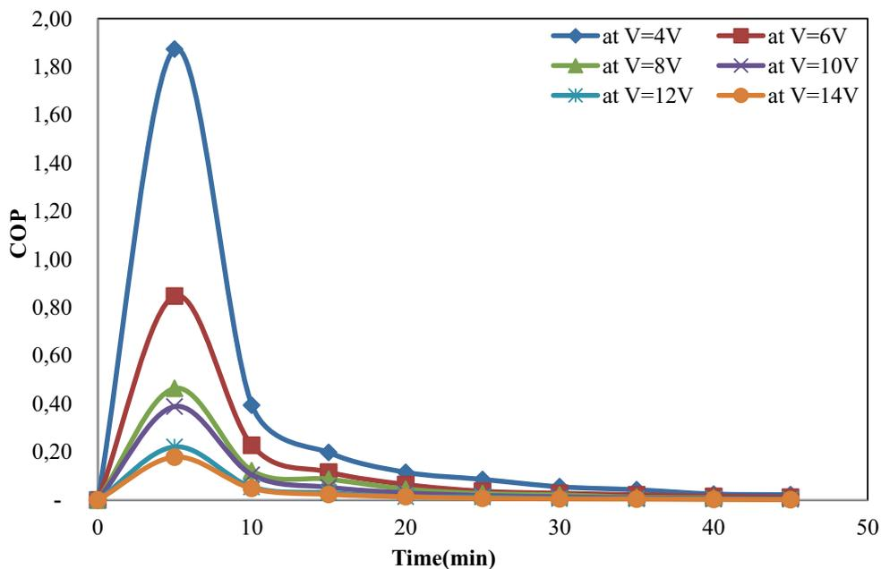
c) Effect of using three Peltier units on COP over time at different voltage
