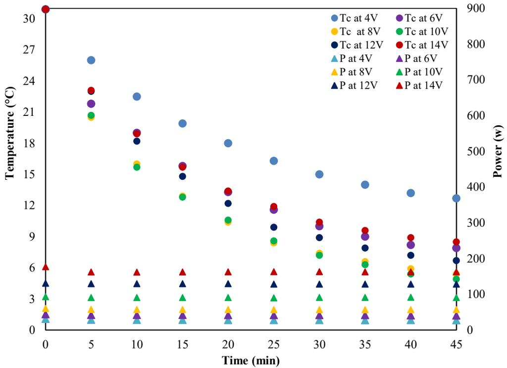
Fig. 10. Temperature and power variations over time for operation with four Peltier units
