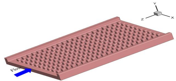
Fig. 1. Isometric view of micro pin fin heat sink.
