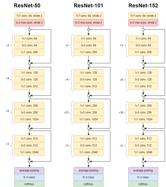
Fig. 6. Visualization of the ResNet-50, ResNet-101 and ResNet-152 architectures
