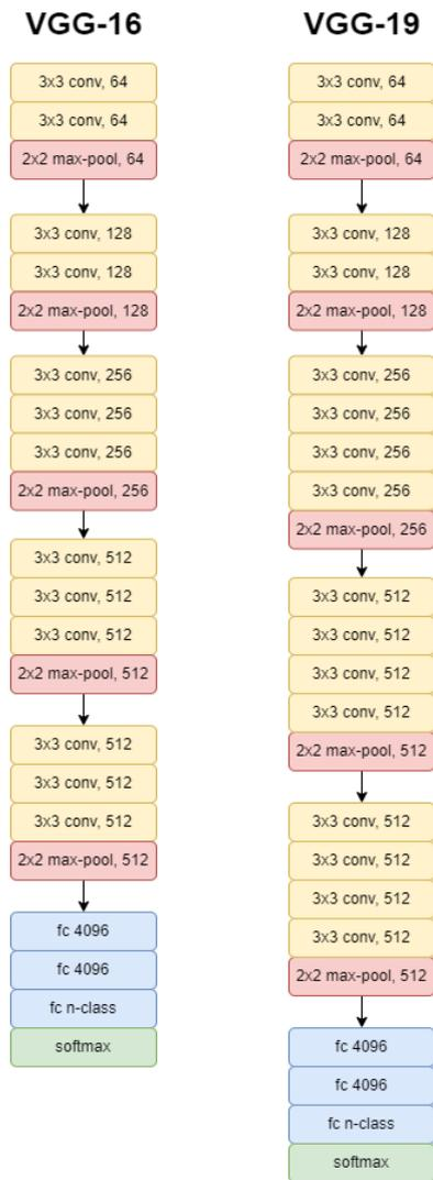
Fig. 5. Visualization of the VGG-16 and VGG-19 architectures
