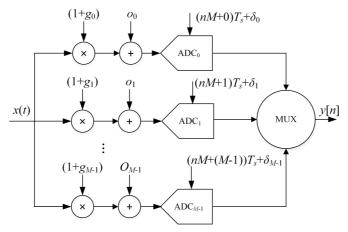
Fig. 1. Diagram of the channel mismatch model.
