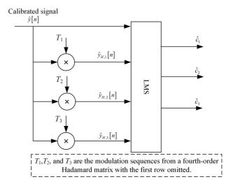
Fig. 4. The diagram of the parameter estimation module of a four-channel TIADC.
