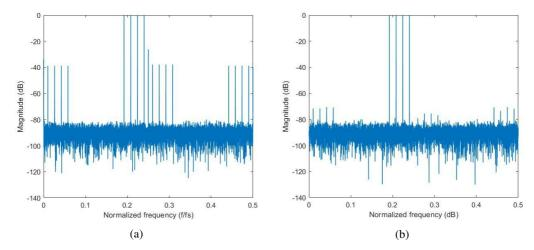
Fig. 7. Calibration performance of the four-channel TIADC (multi-tone signal), a) is the uncalibrated signal spectrum, and b) is the spectrum of the calibrated signal.
