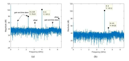
Fig. 9. 4 GHz single-tone signal calibration performance, a) is the uncalibrated signal spectrum, and b) is the spectrum of the calibrated signal.
