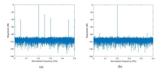
Fig. 5. Calibration performance of a four-channel TIADC (single-tone signal), a) is the uncalibrated signal spectrum, and b) is the spectrum of the calibrated signal.
