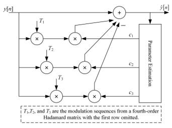
Fig. 3. Calibration structure of a four-channel TIADC.
