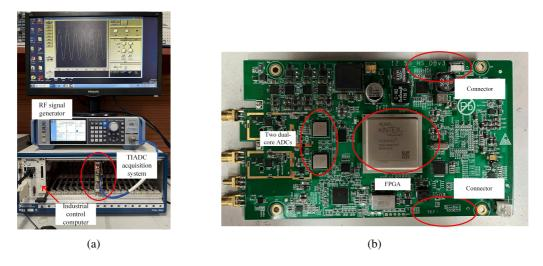
Fig. 8. 12.5 GSPS four-channel TIADC system hardware platform, a) is the whole acquisition system, and b) is the prototype of the acquisition system.
