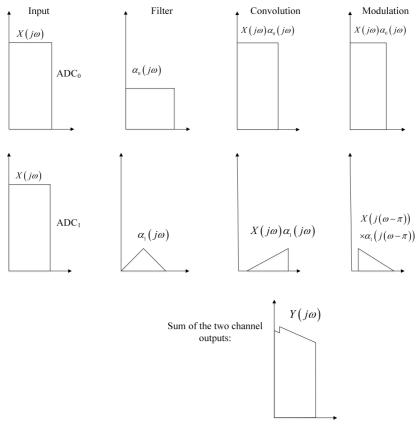
Fig. 2. Example of a two-channel system output.
