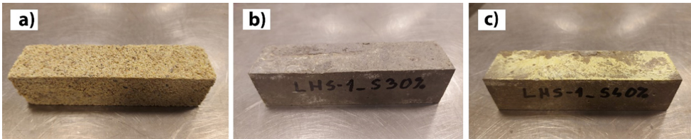
Fig. 2. Specimens made of sulfur concrete: a) SC_S20 (sand and 20% of sulfur), b) SC_LHS40 (lunar simulant LHS-1 and 30% of sulfur), c) SC_LHS40 (lunar simulant LHS-1 and 40% of sulfur)
