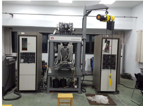
Fig. 3. MTS-816 electro-hydraulic servo triaxial testing machine
