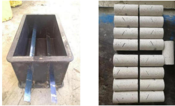
Fig. 1. Test mold and rock-like specimens with joints
