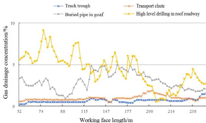
Fig. 13. Variation law of gas drainage concentration with working face advancing
