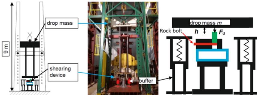
Fig. 12. The single shear impact test rig [36]
