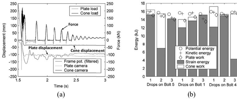
Fig. 15. (a) the force and displacement measured versus time during the impact tests [40] and (b) the comparison of different energy states in the dynamic tests (In all tests, the drop weight and mass were 1461 kg and 1 m, respectively) [42]
