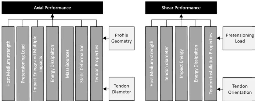
Fig. 13. The parameters which their effects on tendon behaviour were examined under impact loading mode
