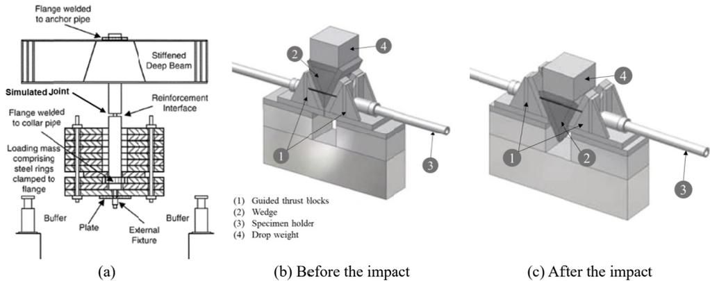
Fig. 6. (a) the WASM impact test rig, adapted from [22,11], (b) and (c) the SRK/Duraset wedge-block loading device, adapted from [31]
