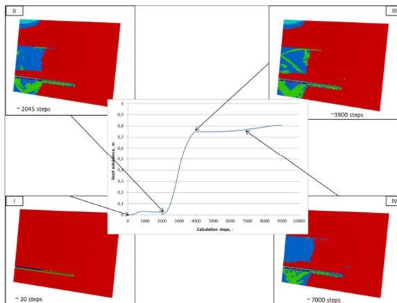
Fig. 11. Convergence and fracture propagation of rock mass in case of 80-m salt layer
