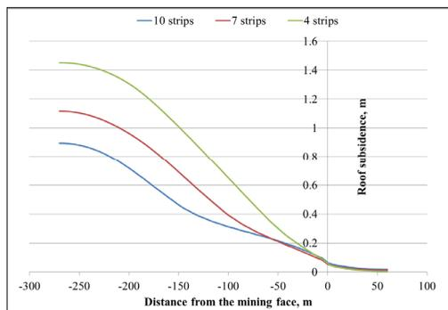
Fig. 12. Roof subsidence along the mining direction with a different width of the opening front (working zone)
