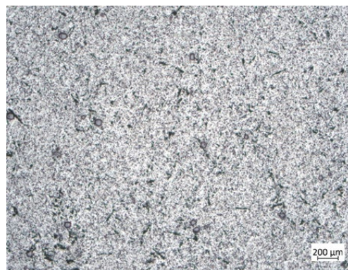
Fig. 6. Microstructure of AlB alloy (25x)
