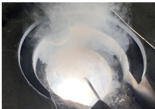
Fig. 5. Intensive evaporation of Mg from the melt
