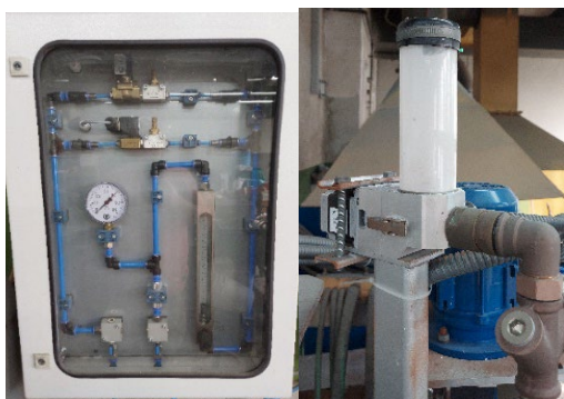
Fig. 2. Refining gas-dispensing system and powder flux dispenser in rotary degassing system
