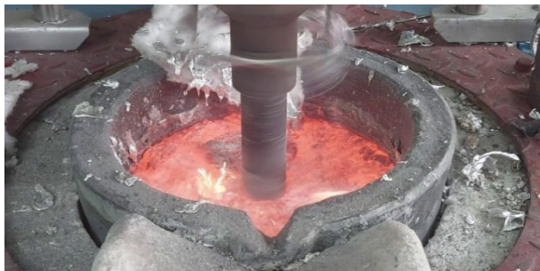
Fig. 5. Effect of introducing powder flux into metal bath – characteristic flare visible on surface of liquid metal
