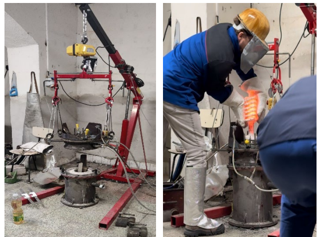
Fig. 6. Experimental LPIC casting machine (left) and attachment of ceramic shell on casting machine (right)
