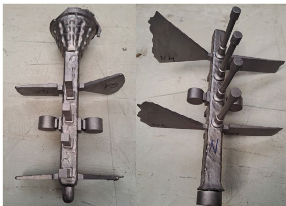
Fig. 7. Casted trees (left: gravity casting, right: LPIC)
