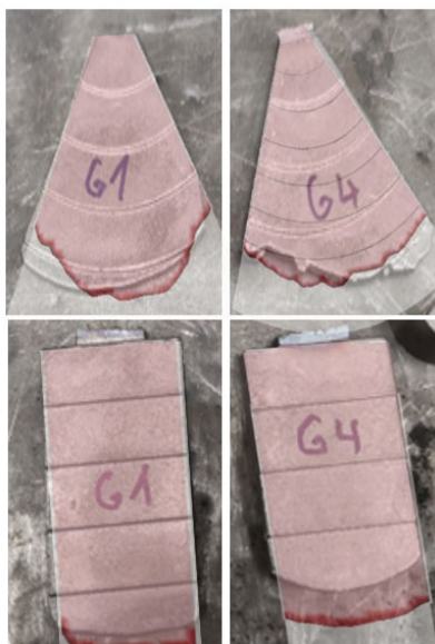
Fig. 13. Comparison of castings with simulation (Gravity casting)
