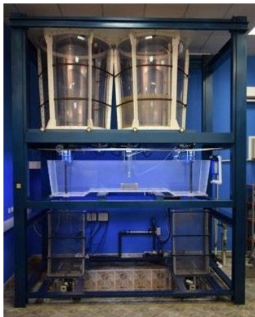
Fig. 2. 0.33 scale water model of two-strand slab tundish
