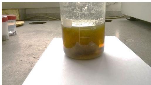
Fig. 5. Reaction mixture after the chemical removal of varnish layers from the tested steel sheet samples
