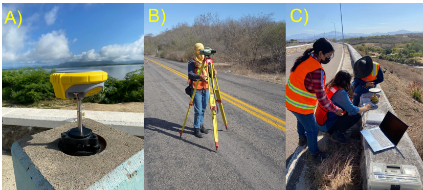
Fig. 3. Equipment used: a) Geodetic GNSS receiver (GEOMAX ZENITH25), b) DNA-03 Leica level, c) Low-cost GNSS receiver, model ZED F9P with antenna ASTECH701975.01A
