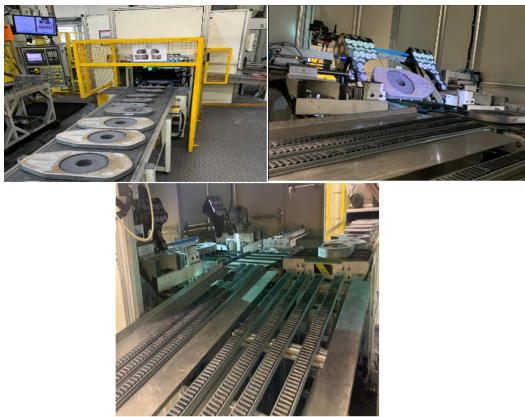
Fig. 10. A production belt directing the plates into the camera
