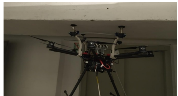
Fig. 14. Drone after docking to the surveyed surface
