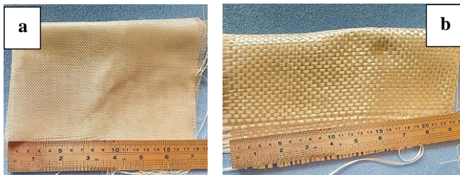
Fig. 4. Glass fiber composite material. (a) 200 g/m 2 glass fibers, (b) 300 g/m 2 glass
