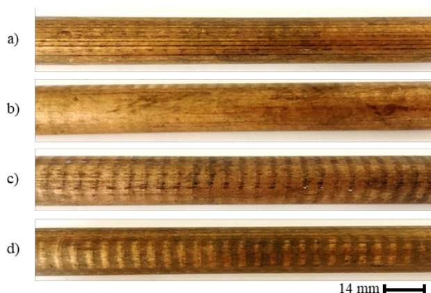
Fig. 4. View of rods obtained via the continuous casting process (a) CuSc0,1, (b) CuSc0,2, (c) CuSc0,3, (d) CuSc0,4
