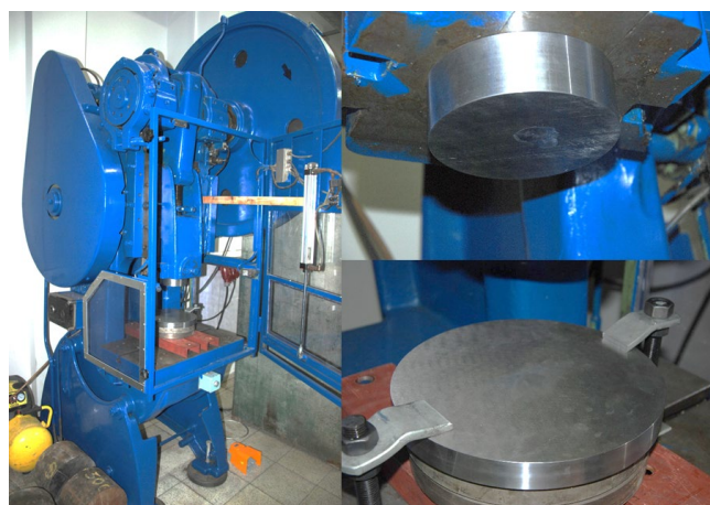
Fig. 5. View of eccentric press (max. force 40kN) with flat die
