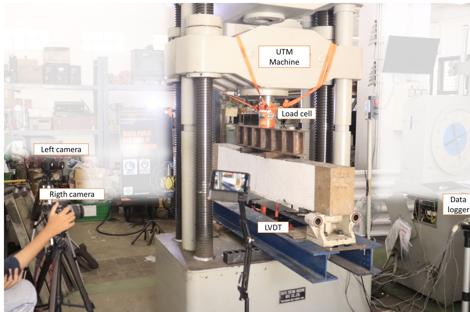
Fig. 5. Beam test set up for four-point load bending
