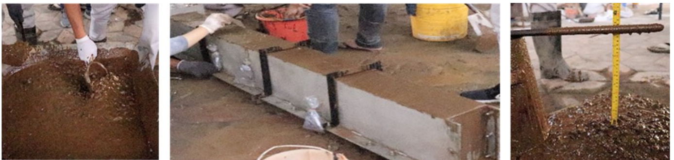
Fig. 4. Casting process and slump test of beam specimens
