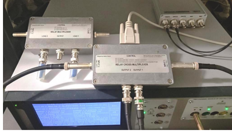
Fig. 3. Photograph of cross multiplexer. The old single-output version of the MUX with external loads is visible on the top left.
