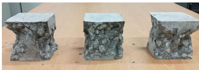
Fig. 5. Pattern of failures for APWP concrete
