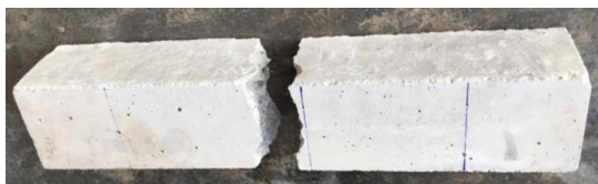
Fig. 7. Pattern of failures for APWP concrete beam
