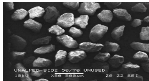
Fig. 4. Morphology of quartz particles used in abrasion tests
