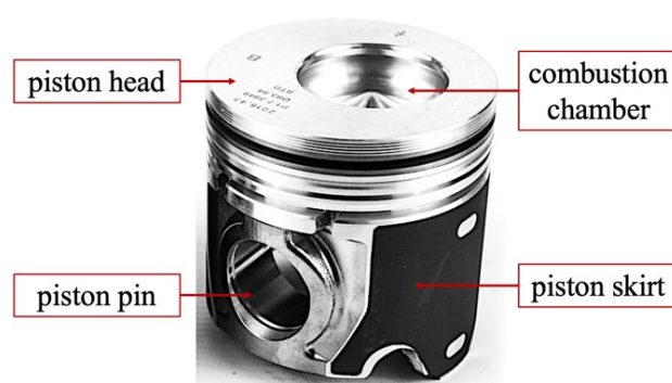
Fig. 1. View of the AlSi12CuNiMg combustion engine piston made by PMC
