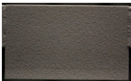
Fig. 7. Surface appearance of the ZrO 2 -Y 2 O 3 coating on AlSi7Mg alloy casting after APS spraying
