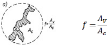
Fig. 8. Scheme of shapes of graphite precipitate cross-sections [8]
