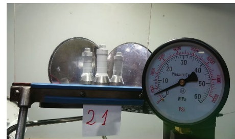
Fig. 20. System of mirrors for tracking surfaces of samples from three sides in real time
