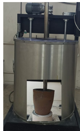
Fig. 1. Visual of steel rod in induction furnace and crucible used in casting
