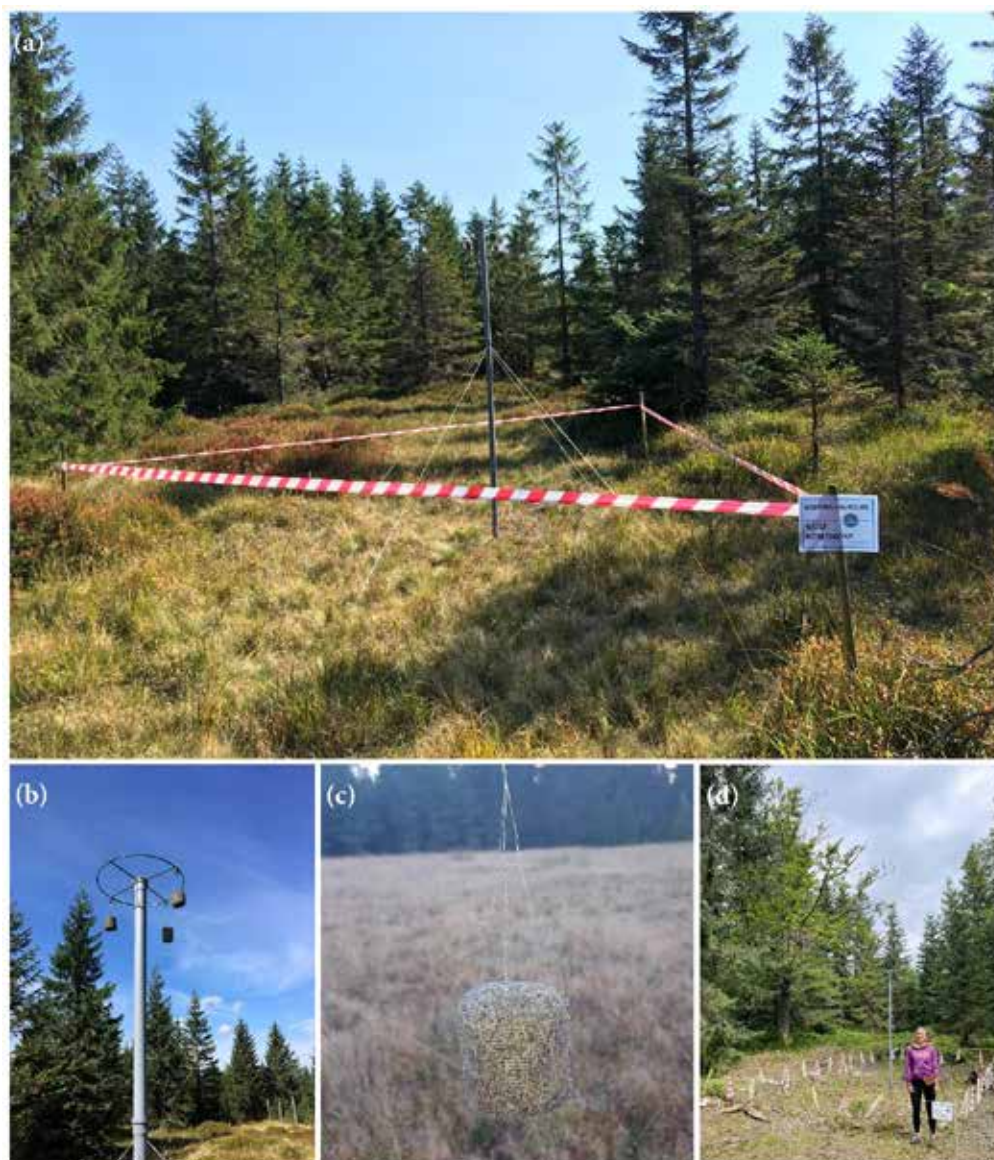
Figure 1. Photographs: (a) research installation on research plot in the spring–summer season (near the “Kobyła” hill, Izery Mountains), (b) fragment of the installation with moss bags (during the exposition cycle) in the spring–summer season (near the “Kobyła” hill, Izery Mountains), (c) moss bag (during the exposition cycle) in the spring–summer season (in the “Orle” forest glade, Izery Mountains), and (d) research installation on research plot in the spring–summer season (near the “Granicznik” hill, Izery Mountains)
