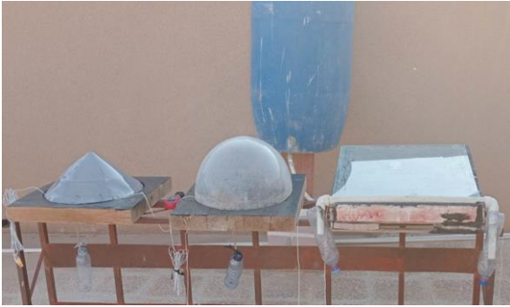
Fig. 4. Photograph of the full experimental setup showing the placement of the three solar still types (single-slope, hemispherical and conical) under identical outdoor environmental conditions.
