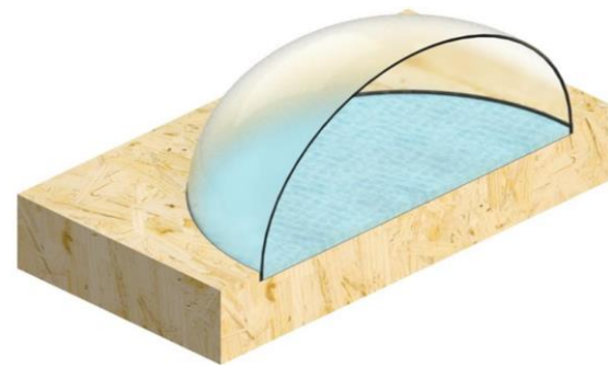
Fig. 1. Schematic representations of the hemispherical solar still design used in the experimental setup, highlighting geometric configuration, materials and insulation layout.
