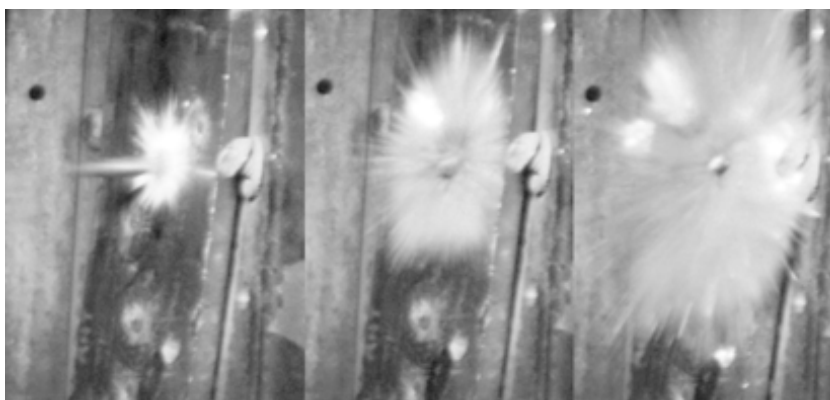
Fig. 17. 7.62 \times 39 mm FMJ PS bullet stopped by an armored plate
