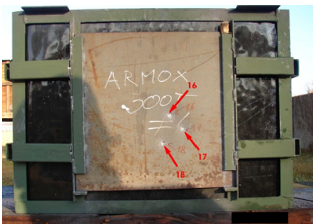
Fig. 9. Fuel tank covered with A500T fired with a 7.62 \times 39 mm FMJ PS projectile Kalashnikov – shots 16–18
