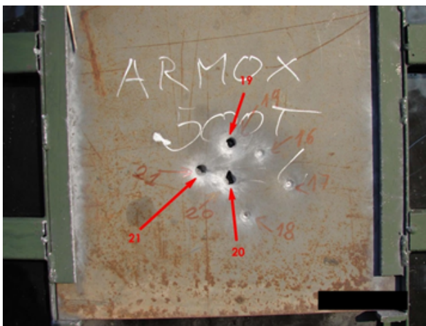
Fig. 10. Fuel tank covered with A500T tested with .308 WIN Match bullet – shots 19–21
