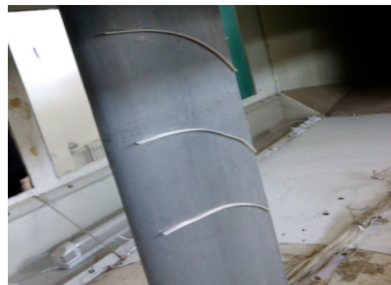
Fig. 4. Experimental model of blade guide bar pressure measurement
