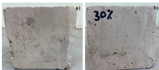
Fig. 6. The samples after exposed to fire resistance a) 10 CBA at 800°C b) 30 CBA at 800°C
