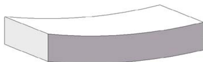
Fig. 3(c). Plate shape warping of the strip steel after instability
