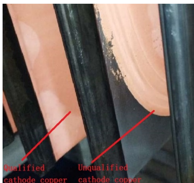
Fig. 8. Different morphologies of cathode copper products after electrolysis
