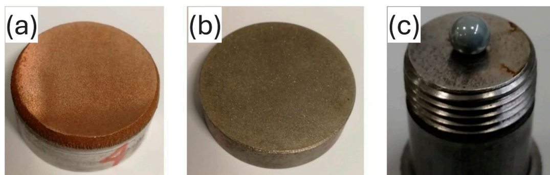
Fig. 12. Samples for testing: (a) DMMC, (b) D30, and (c) \text{Si}_3\text{N}_4 ball [38]
