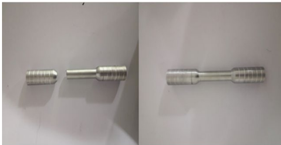
Fig. 2. Tensile Test Samples Before And After Fracture
