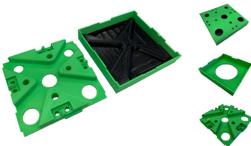
III. 7. Casting mold. The final mold after mechanical processing is shown on the right. Author Wojciech Kocki.
