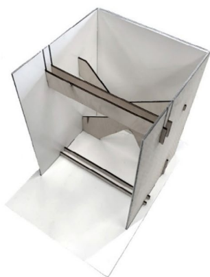
III. 6. The fabrication process of the remaining part of the casting module, laser CNC. Author Wojciech Kocki.
