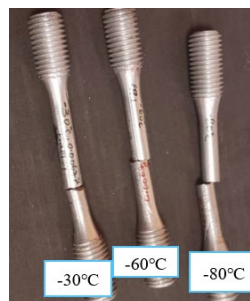
Fig. 12. Failure state of EN AC-Al Si12CuNiMg aluminium alloy at different low-temperature
