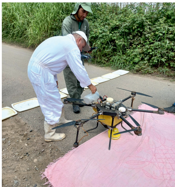
Fig. 2. Using the trays to determine distribution of drone granule rate
