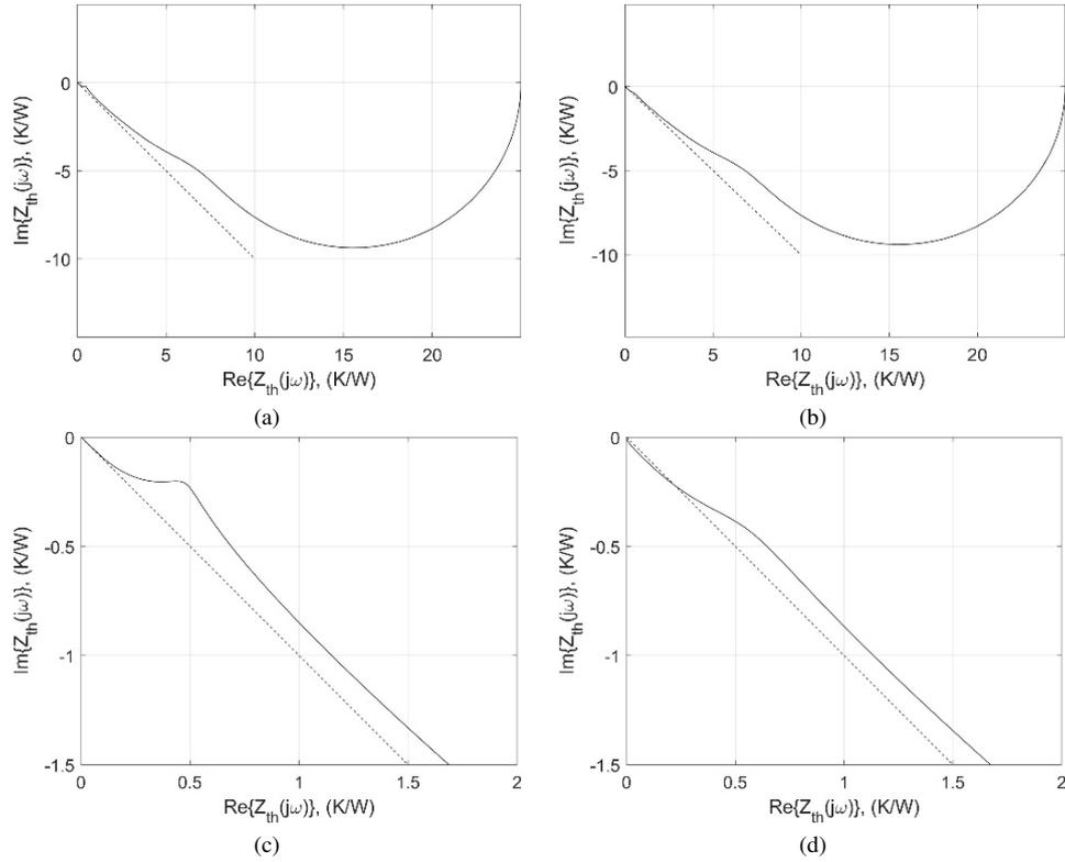
Fig. 13. Results comparison of analytical (a) and  $R_{th}C_{th}$  ladder DPL diffusive model (b) –  $\tau_T = 2$  s,  $\tau_q = 10$  s,  $\text{err} = 5.92\%$ . Subfigures (c) and (d) show a zoomed view of a higher range of frequencies, respectively
