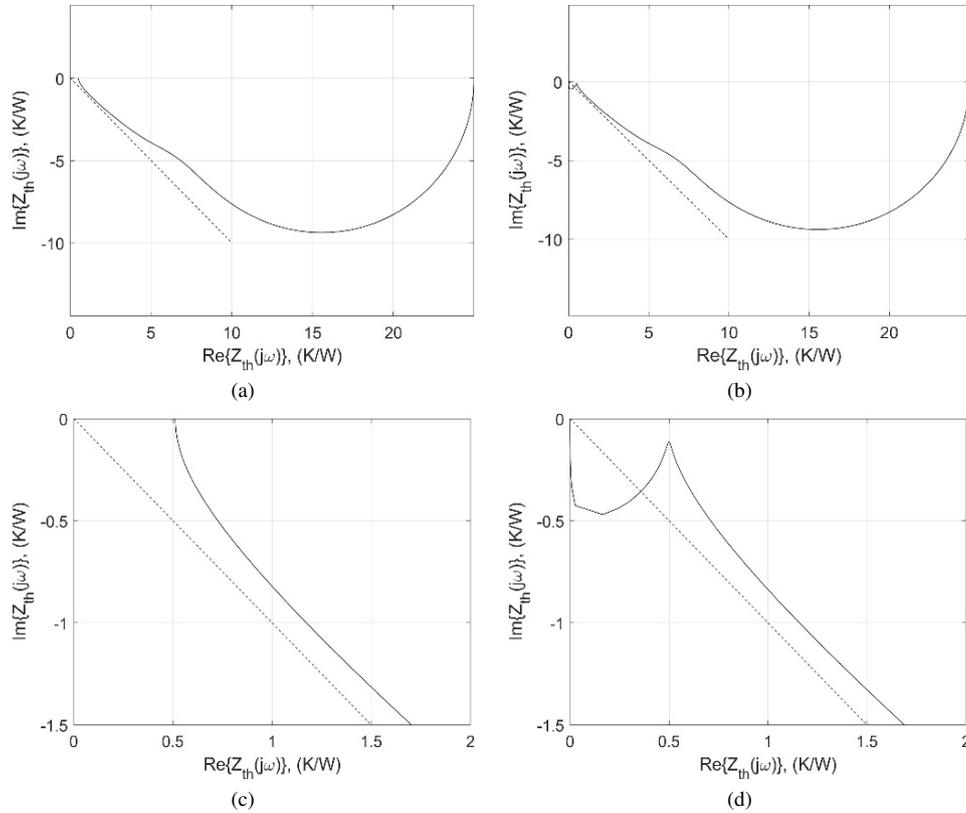
Fig. 12. Results comparison of analytical (a) and  $R_{th}C_{th}$  ladder DPL wave model (b) –  $\tau_T = 0$  s,  $\tau_q = 10$  s, err = 1.8%. Subfigures (c) and (d) show a zoomed view of a higher range of frequencies, respectively
