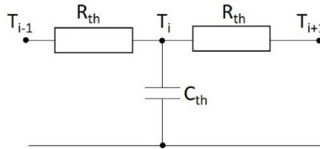
Fig. 2. Thermoelectric analogy circuit of Fourier–Kirchhoff’s heat conduction
