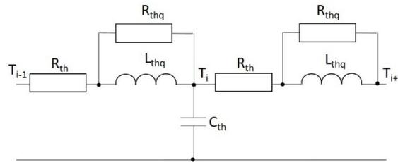
Fig. 6. Thermoelectric analogy circuit of DPL heat conduction for  $\tau_q > \tau_T$
