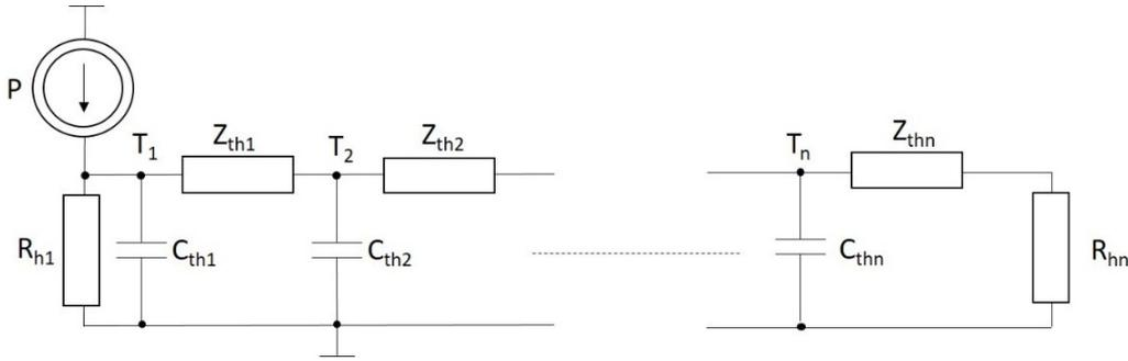
Fig. 8. Thermal ladder model of an object with DPL effects
