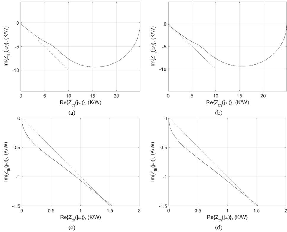
Fig. 10. Results comparison of analytical (a) and  $R_{th}C_{th}$  ladder SPL model (b) –  $\tau_T = 10$  s,  $\tau_q = 0$  s,  $\text{err} = 0.65\%$ . Subfigures (c) and (d) show a zoomed view of a higher range of frequencies, respectively
