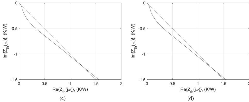
Fig. 11. Results comparison of analytical (a) and  $R_{th}C_{th}$  ladder DPL diffusive propagation model (b) –  $\tau_T = 10$  s,  $\tau_q = 2$  s,  $\text{err} = 0.7\%$ . Subfigures (c) and (d) show a zoomed view of a higher range of frequencies, respectively
