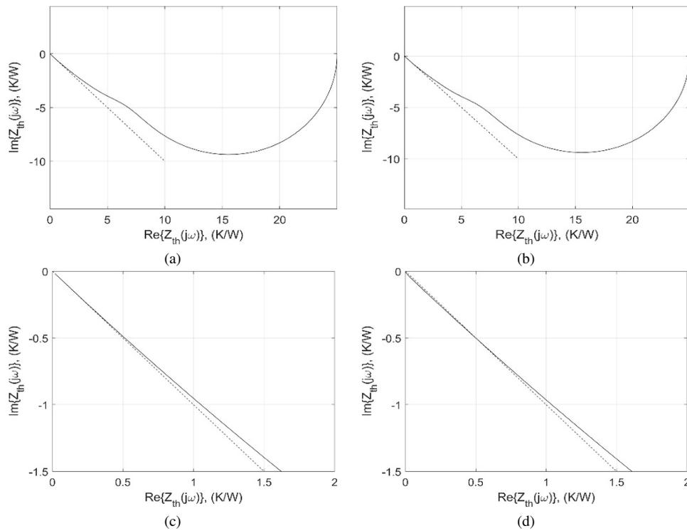
Fig. 9. Results comparison of analytical (a) and  $R_{th}C_{th}$  ladder Fourier-Kirchhoff's model (b) -  $\tau_T = 0$  s,  $\tau_q = 0$  s, err = 0.99%. Subfigures (c) and (d) show a zoomed view of a higher range of frequencies, respectively
