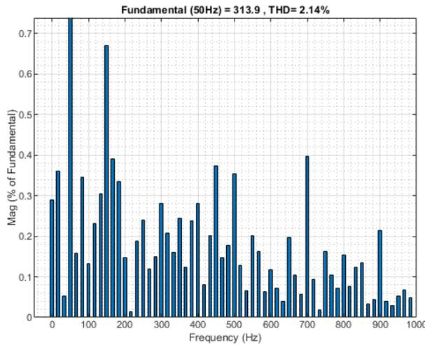
Fig. 10. Frequency spectrum of load voltage (FFT analysis)
