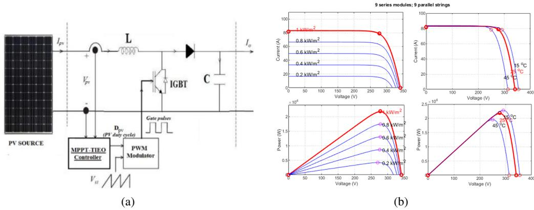
Fig. 2. (a) Synoptic diagram of the PV source integrated with a boost converter; (b) photovoltaic module characteristic (I-V and P-V curves)
