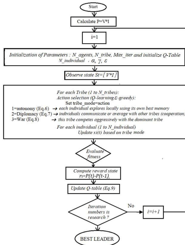
Fig. 4. Flowchart of the proposed TIEO-MPPT algorithm
