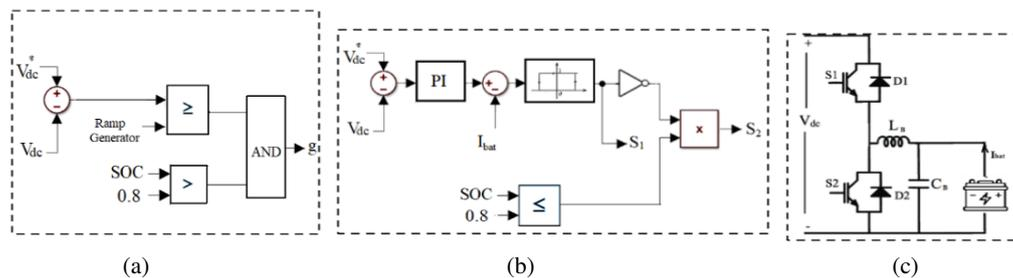
Fig. 5. (a) The schematic diagram of dump load controller; (b) SE-DC-link voltage controller via (c) DC-DC bidirectional converter
